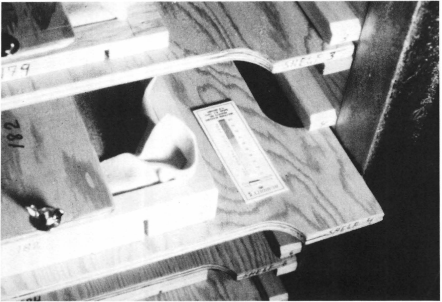
4. Humidity Indicator Cards in tray of silica gel checks RH of buffer.
